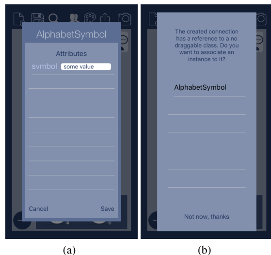
Figure 9: (a) Creating an instance of a class. (b) Associating that instance to a connection.
