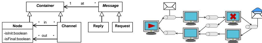
Fig. 2. The DSL meta-model (left). A model (right).
